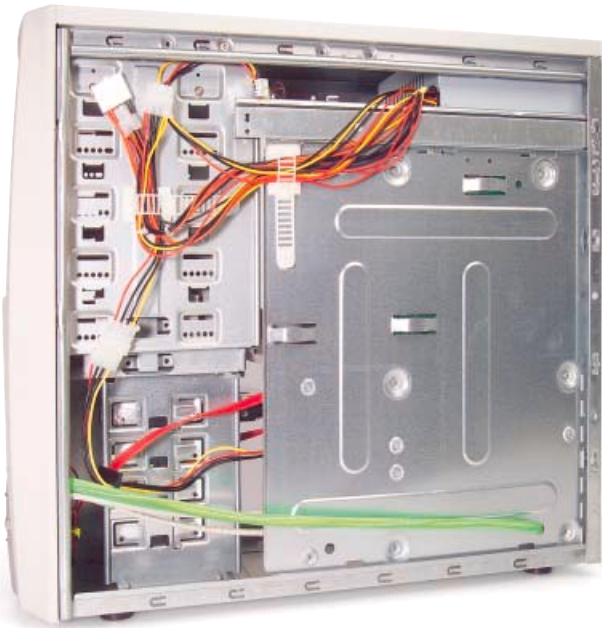
Adjustable ties make light work of keeping wires and leads in order
